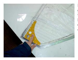
Lay the sail on the table with its head on the gauge (see pic left). The gauge helps to check the width of the headboard, depth of the headboard and primary reinforcement, location of the Aft Head Point and the distance from the 425 mm Upper Leech Point to the luff.
