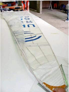
Mark the leech points at leach (see pic below). Check the widths. Check concavities on the leech and sail reinforcements.
