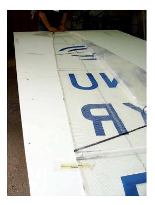
For checking the battens it is practical to use narrow batten with batten lengths marked on it. It is not necessary to remove battens from the pockets when measuring its length and leech length. Check batten pockets and sail corners.
